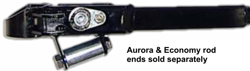
Roller is angled so sway bar rides squarely on arm when front end drops
