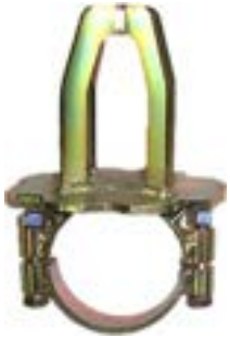
3110-XL – Clamp on Extended Spring Seat – Meets IMCA spring height rule. Spring guide is 4.0" tall to help retain LR spring when "hiked up."
